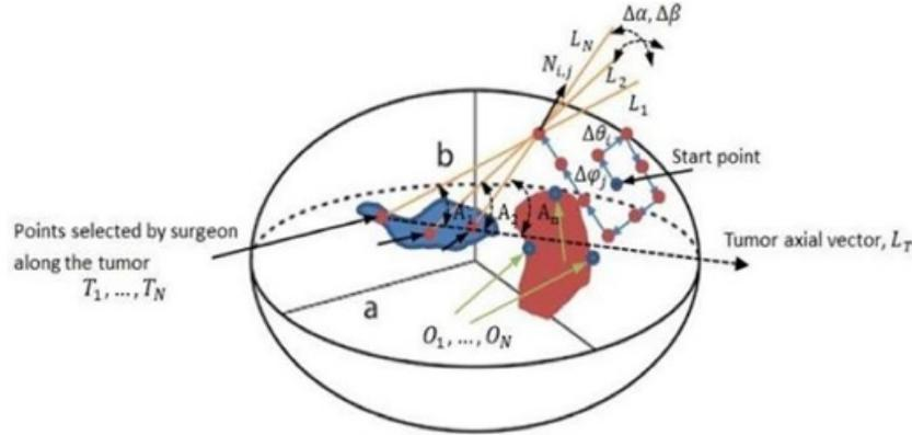
Figure 2 Diagram of proposed search algorithm concept which searches along the skull surface with  $\Delta\theta$  and  $\Delta\varphi$  steps while minimizing the angle between  $L_T$  and  $\{L_1, \dots, L_N\}$
