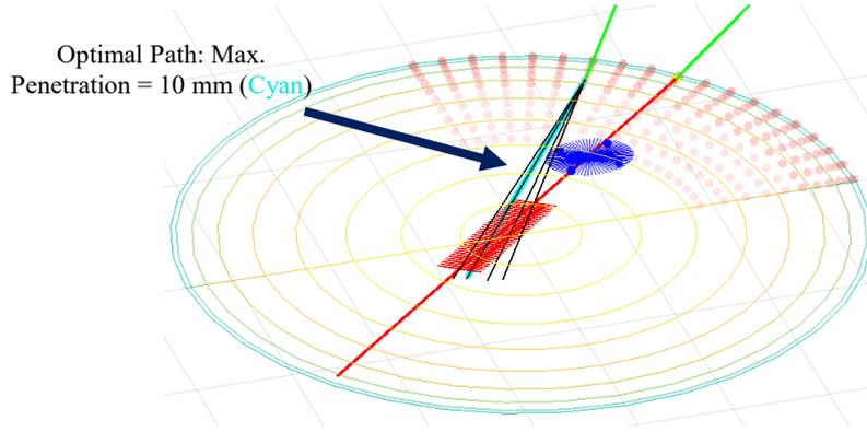
Figure 4 MATLAB model depicting top view of electrode orientations passing through tumor, avoiding obstacle and selection of optimal path
